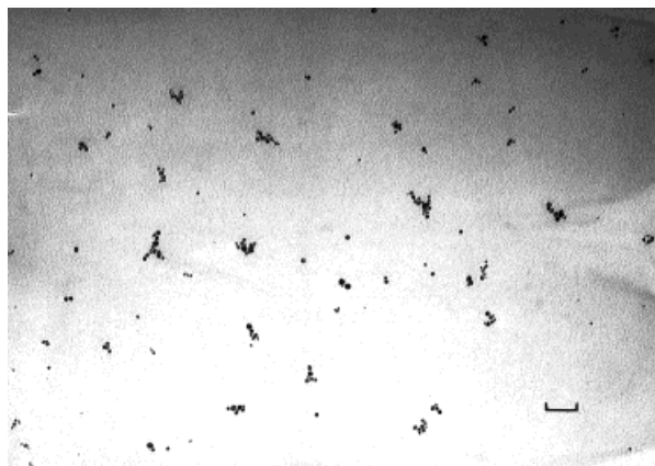
Figure 1 Palladium nanoparticles reduced from \text{PdCl}_2 in the presence of poly(styrene sulfonic acid) (bar = 47 nm).
